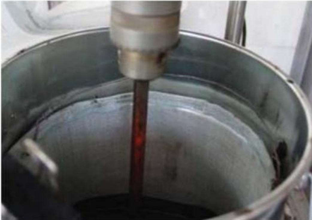
Figure 1. Production of the asphalt-rubber binder.
